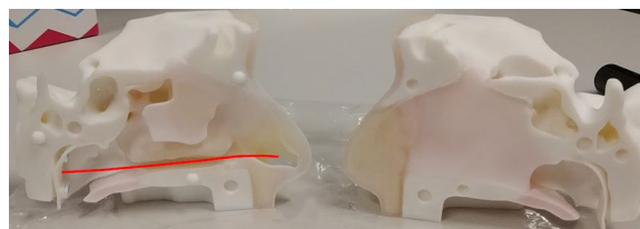
Fig. 4. Nasal cavity phantom used for validation experiments. The red line highlights the path to reach the nasopharynx from the nostril.
