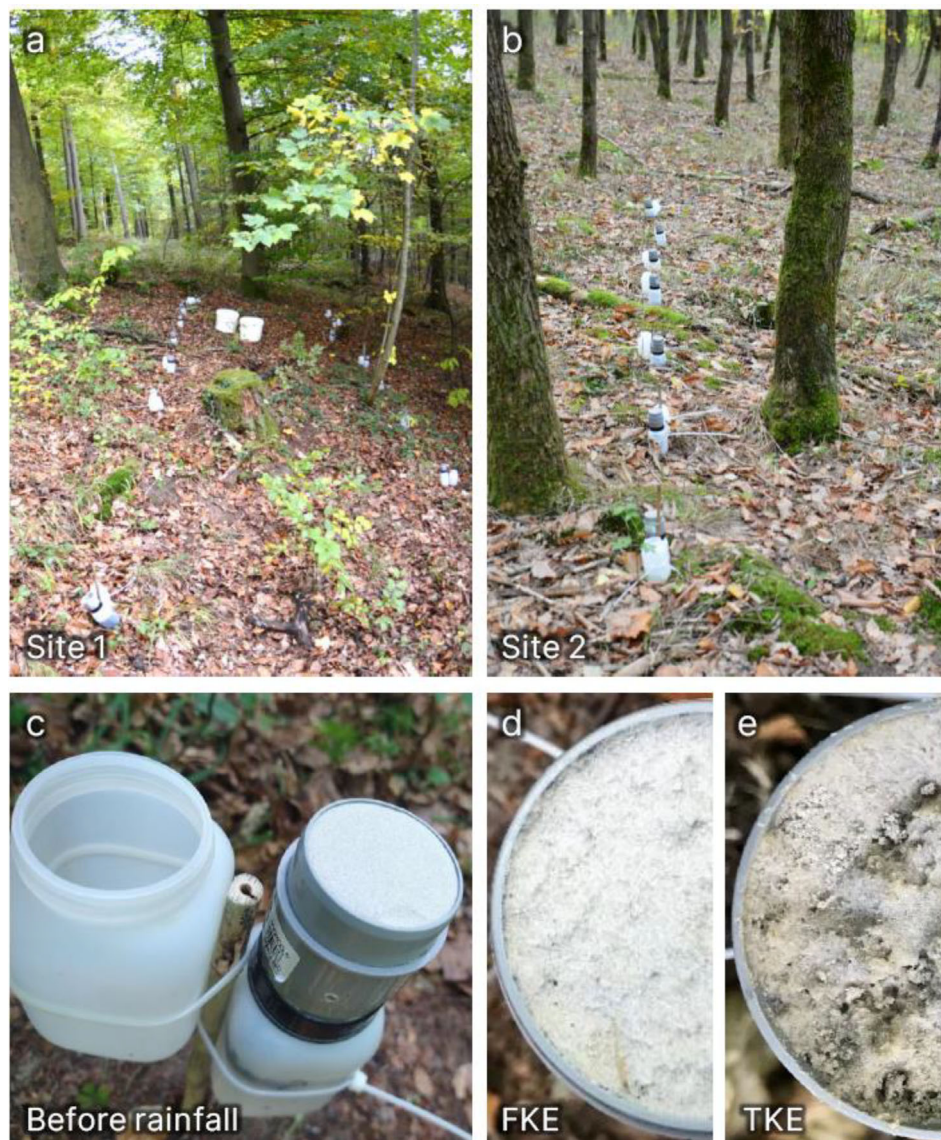
FIGURE 2 Measurement transects and vegetation on Site 1 (a) and Site 2 (b) with an exemplary splash cup before a rainfall event (c) and after a rainfall event without forest canopy (d: FKE) and with closed forest canopy (e: TKE).
