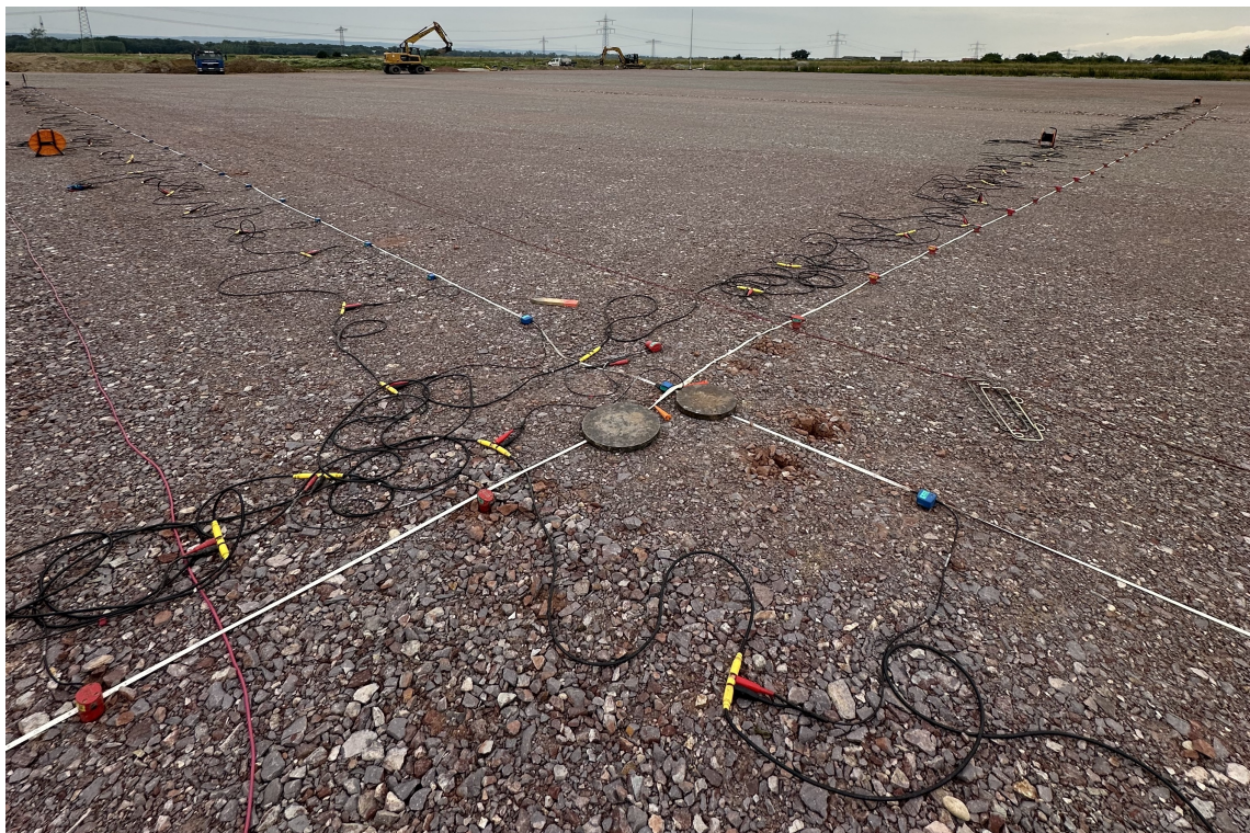
Figure 4.4: MASW field acquisition configuration at the Herrenknecht test site (Photograph by the author).
