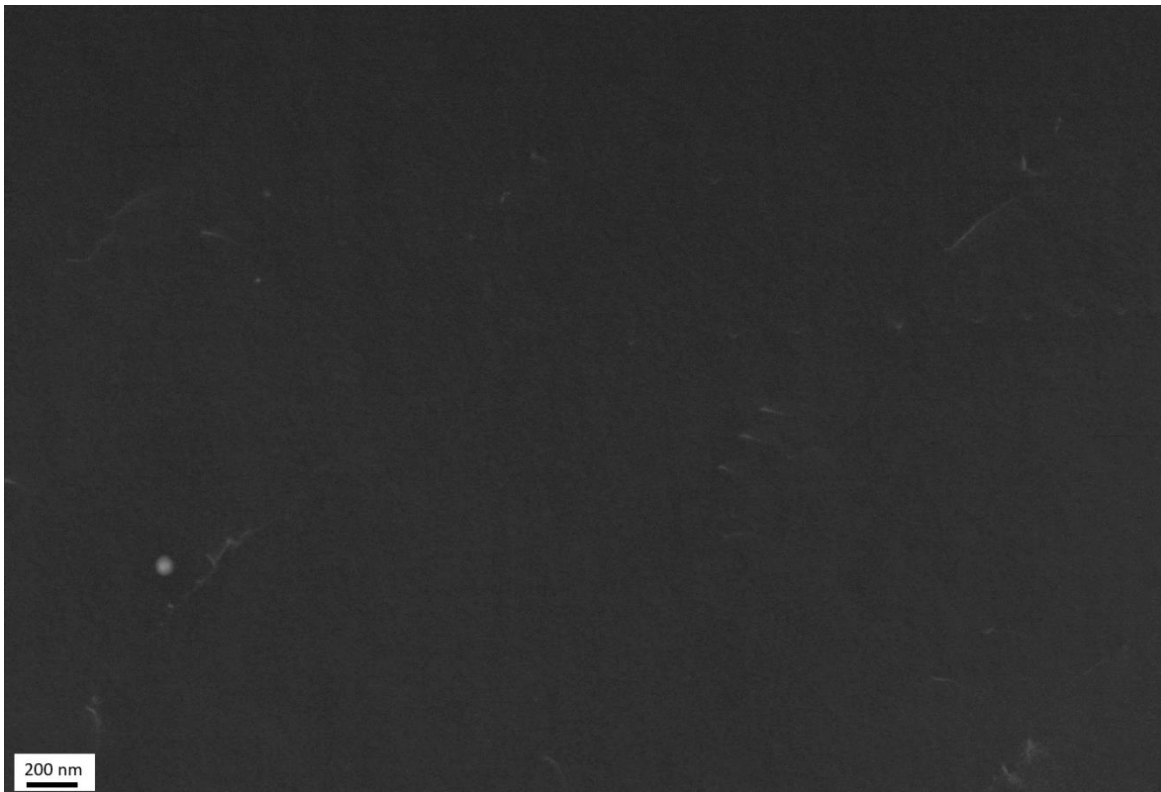
Figure 9-1 SEM ECCI analyses to calculated initial dislocation density by the line intersection method (reprinted from [9]).
