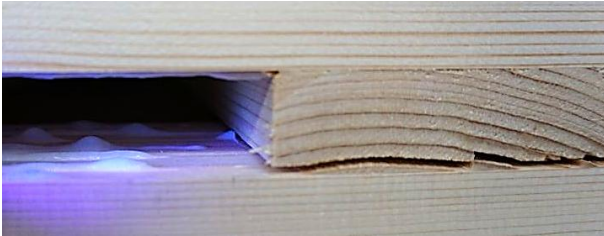
Figure 3. Offset of adhesive application
