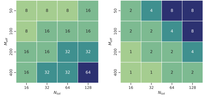
Figure 9: Optimal distribution of resources for different combinations of M_{eff} and N_{tot} . Left: Optimal number of parallel chains. Right: Optimal number of threads for prefetching.
