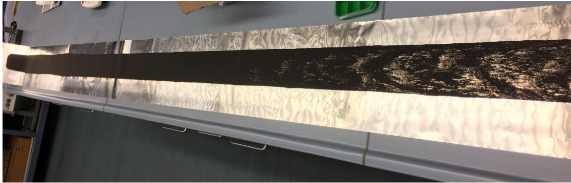
Figure 9. Image of a coated NMC622 cathode on an aluminum current collector, taken immediately after casting and drying, illustrating variations in coating quality along the coating direction. On the left side, corresponding to the initial stages of coating, a uniform and defect-free layer is observed, attributed to favorable slurry rheology. In contrast, on the right side, significant coating defects become evident, resulting from rapid slurry gelation that hindered continuous processability during the coating of the additive-free A 70 wt.% SC cathode slurry.
