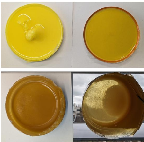
Figure 81. Pictures of vinylogous urethane materials. Top: VU2 before (left) and after drying in oven 80°C (right). Bottom: VU3 before (left) after two weeks at rt (right).
