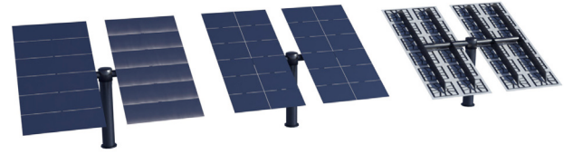
Fig. 1. Visual representation of the heliostat geometries used in our study. From left to right: 2 \times 6 collector, 4 \times 6 collector and the backside of the 4 \times 6 collector. Exemplarily, the right side of the 2 \times 6 collector is shown with soiling on the mirror facets.
