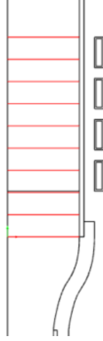
Figure 10. Cutlines at which the plasma parameters are calculated. The lowest is numbered 1, while the highest is numbered 10.
