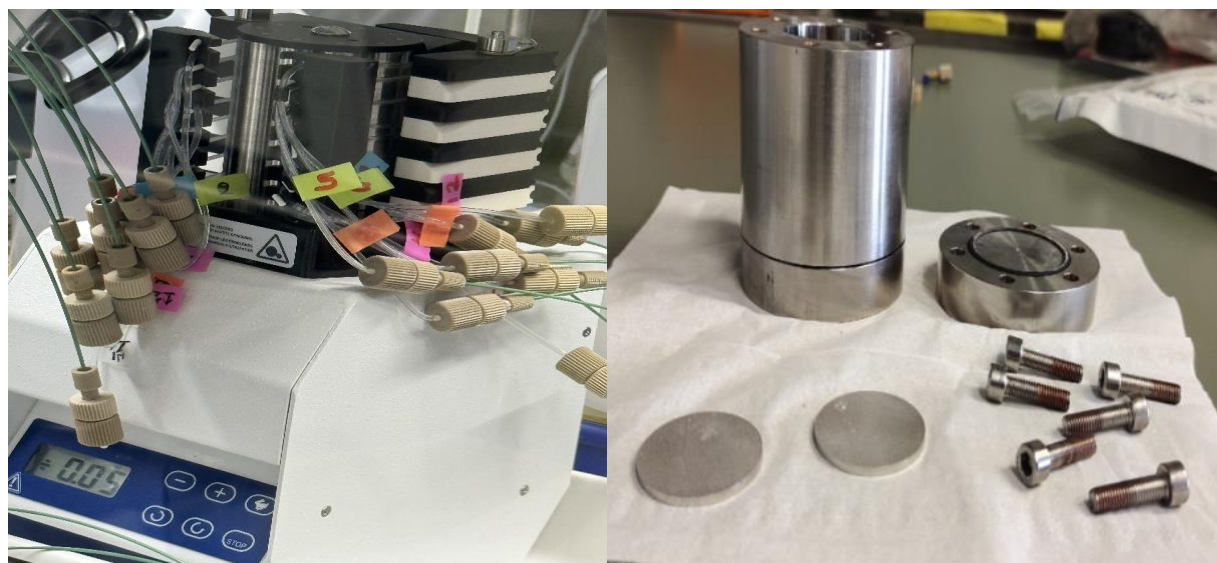
Figure 10 Peristaltic pump on (left side) and reactor set up on (right side) for dynamic experiments.
