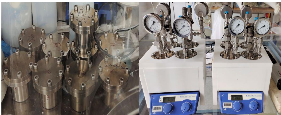
Figure 9 Static experiments on the left at 25°C and right side at 50 °C for 3 and 6 months.
