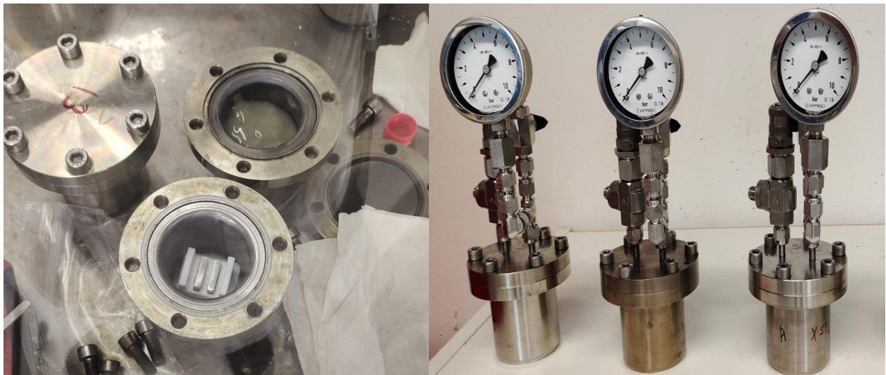
Figure 8 The autoclaves setup with fittings (left) for 25°C and (right) side for 50 °C for static experiments.
