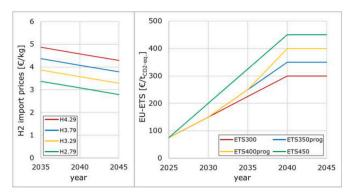
**Fig. 8.** Variations of hydrogen import prices (left) and EU-ETS prices (right), that are combined with each other to identify conditions for accelerated defossilization pathways.
