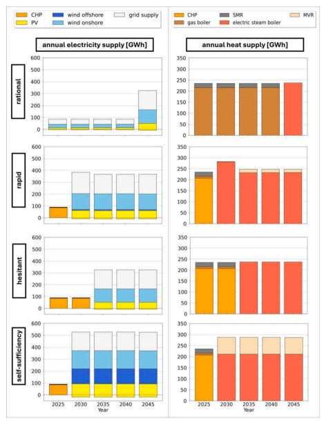
Fig. 5. Scenario results regarding the industrial site's electricity and heat supply. Note: Surplus electricity is shown negative. Although it may appear so, surplus electricity stems not necessarily from PV.
