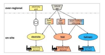
**Fig. 1.** Schematic of the site's current energy and hydrogen system, focusing on the key components and interfaces pertinent to the study.
