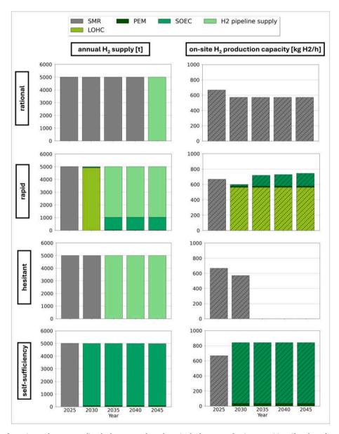
Fig. 3. Cost-optimal transformation pathways regarding hydrogen supply and on-site hydrogen production capacities. Clear bars denote values associated with flows, while hatched bars denote values associated with capacities.
