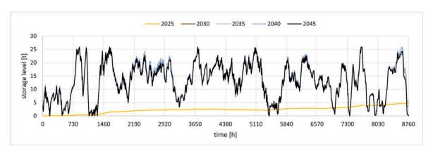
Fig. 4. Hydrogen storage level in the self-sufficiency scenario. Note: The curve of 2045 mostly overlaps the curves of 2030, 2035 and 2040.
