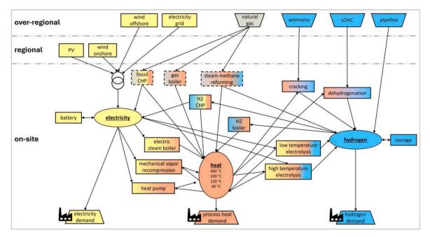
Fig. 2. Modeled system and its included technology options, differentiated by its location. Dashed squares represent technologies that are already in place nowadays. Colors represent the respective sectors of the industrial site: yellow for electricity, orange for process heat, and blue for hydrogen. (For interpretation of the references to colour in this figure legend, the reader is referred to the Web version of this article.)
