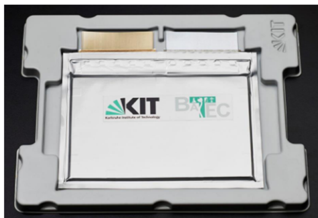
Figure 3. Target pouch cell format with a maximum cell stack of 6 mm. Here, a LIB is displayed.
