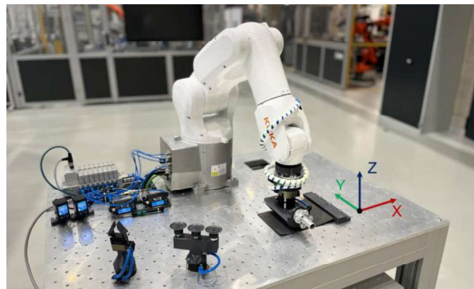
Fig. 1. The semi-automated disassembly setup has a universal kinematic and a six-axis force-torque sensor as main components. The chosen stationary frame of reference is shown as a coordinate system.
