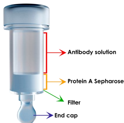
Figure 3-1: The scheme of Protein A HP SpinTrap column. This column utilizes Protein A Sepharose for the purification of antibodies. The column is designed to facilitate the selective binding of immunoglobulin G (IgG) antibodies through the Protein A ligands, allowing for efficient separation from other proteins in a sample. This figure illustrates different parts of the column.
