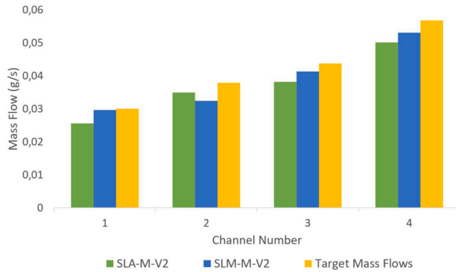
Fig. 7. Comparison between VPP-UVL/P and PBF-LB/M manufactured parts.
