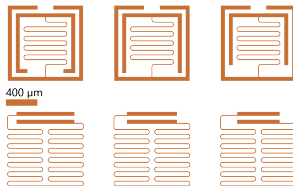
Figure 3.4: Initial resonator designs consisting of horseshoe style (top panel) and meander style (bottom panel) resonators. For horseshoe resonators, the outer capacitor plate was kept constant at 200\mu\text{m} varying the inner capacitor length. For meander resonators, the length of both capacitors was varied. The length of the meander was kept constant in all of them.
