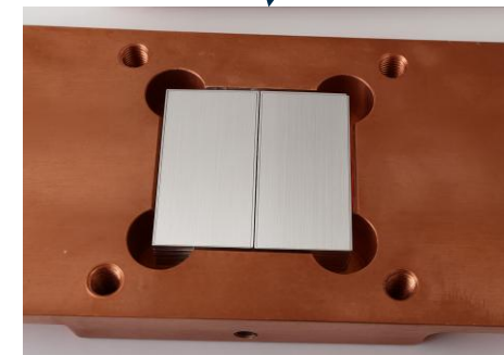
Copper box with HTS tape stack
