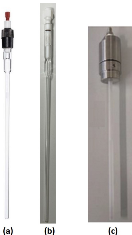
Figure 3.17: Photo of different commercial high-pressure NMR tubes. (a) A 5 mm thin wall quick pressure valve NMR tube (Wilmad-LabGlass). The upper portion of the quick pressure valve is fitted with 1/16 inch PTFE tubing. The maximal pressure is 100 psi. (b) A 5 mm heavy wall NMR pressure tube for medium range pressure ( \leq 300 psi) (Wilmad-LabGlass). The valve is designed to connect to a 1/8 inch tubing using Swagelok ® fittings. (c) A 5 mm sapphire NMR tube for high-pressure ranging up to 200 bar.
