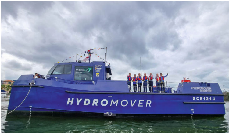
Fig. 4 A photo of the Hydromover, a fully-electric cargo vessel with interoperable swappable battery solution. Source Courtesy Yinson Green Tech (Offshore Energy 2023)
