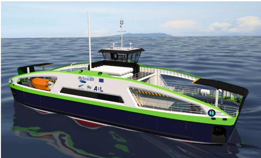
Fig. 8 Rendering of the HySeas III RoPax hydrogen fuel cell RoPax ferry concept. Source Gomez Trillos and Draheim (2022), created by Courtesy of ABL Group/Caledonian Maritime Assets Limited
