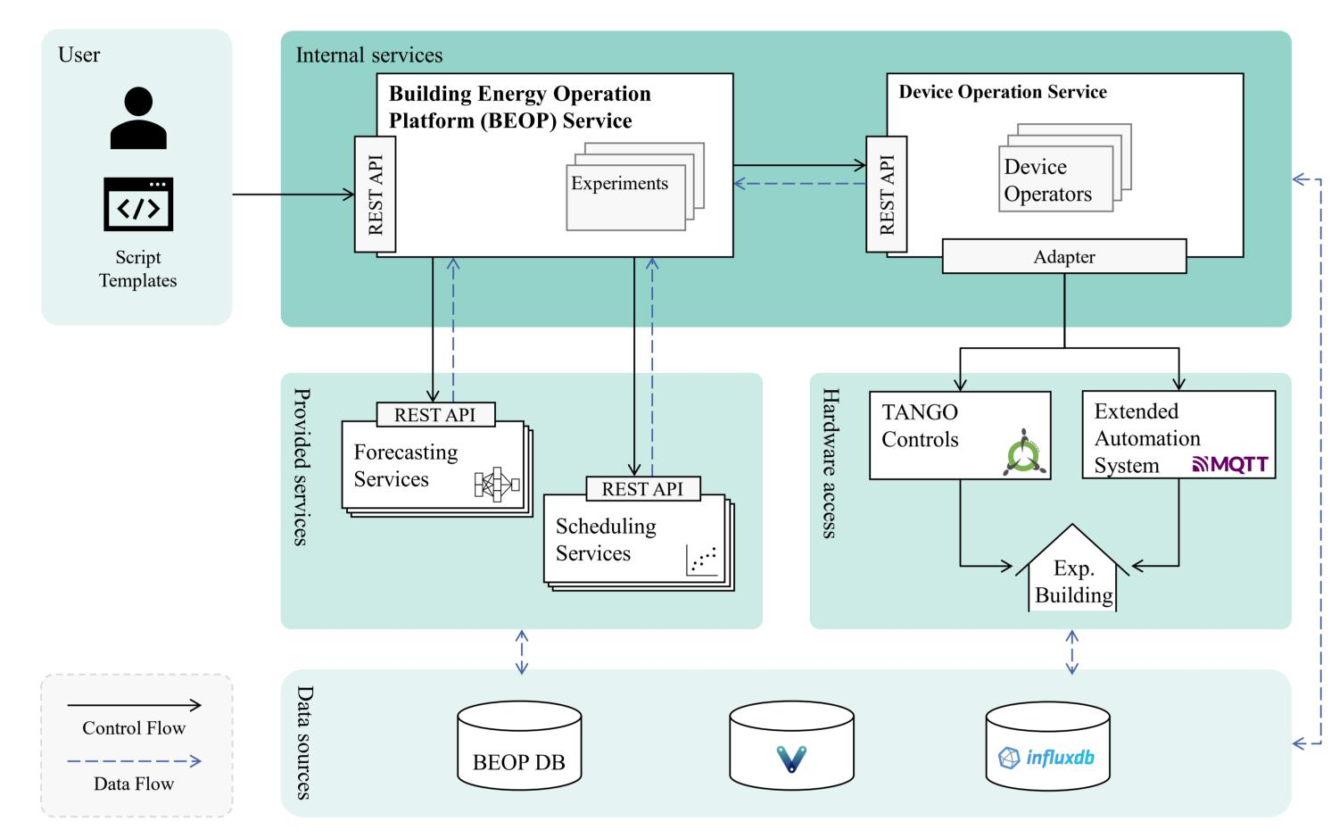
The BEOP core including provided services and interfaces to the real hardware, describing control and data flows.
