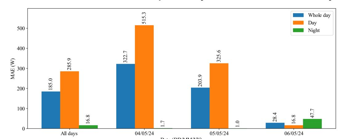
MAE at the PCC, calculated with 10-second resolution. Significant deviations on days one and two when the BESS exceeded capacity, preventing the system from meeting the dispatch schedule.
