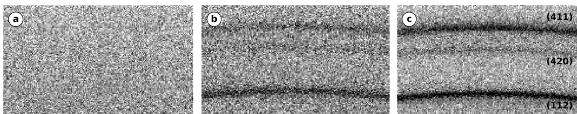
Fig. 1. Selected 2D diffraction frames of \text{Fe}_{40}\text{Ni}_{40}\text{P}_{14}\text{B}_6 recorded in-situ during the 0.67 K/s ramp. (a) Pristine amorphous foil at T = 300 K: the pattern shows only diffuse scattering; no Debye-Scherrer rings are visible. (b) Intermediate stage ( T \approx 707 K): three more or less faint, continuous rings appear, marking the first nucleation of crystalline domains, i.e. onset of crystallisation. (c) Fully crystallised state ( T = 1013 K): bright, sharp Debye-Scherrer rings corresponding to the (112), (420) and (411) reflections of tetragonal \text{Ni}_3\text{P} confirm long-range ordering and grain growth.
