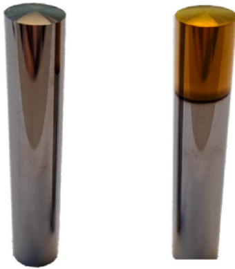
Fig. 5. Pin after grinding (left) and after PVD coating (right).
