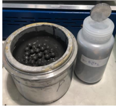
Figure 6.2: Bismuth telluride ink, produced with a ball milling during the production. © 2022 Leonard Franke, reproduced with permission.
