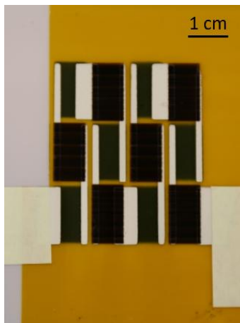
Figure 5.15: Picture of the PEDOT:PSS/PBFDO TEG (6 thermoelements) printed on top of a Kapton substrate after the encapsulation with a 0.7 \mu\text{m} of parylene. Figure from 168 licence CC BY-NC.
