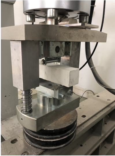
(a) Flexural strength (FS) testing of UHPC specimens prior to halving.
