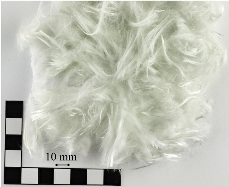
Figure 6.7 Fiber skeleton of a burned plate segment from the center point ( w_{f,mean} = 33\% ) towards the end of the flow path.
