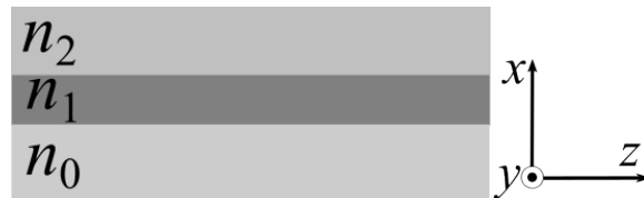
Figure 3.1.: Sketch of a planar waveguide composed of three layers with different refractive indices.
