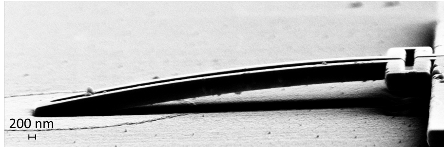
(b) SMA/Si bilayer structure bending down.
