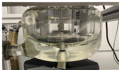
(b) Photo of the experimental setup of the stirred vessel. Besides the ultrasonic probe, also the 6-bladed impeller is visible.
