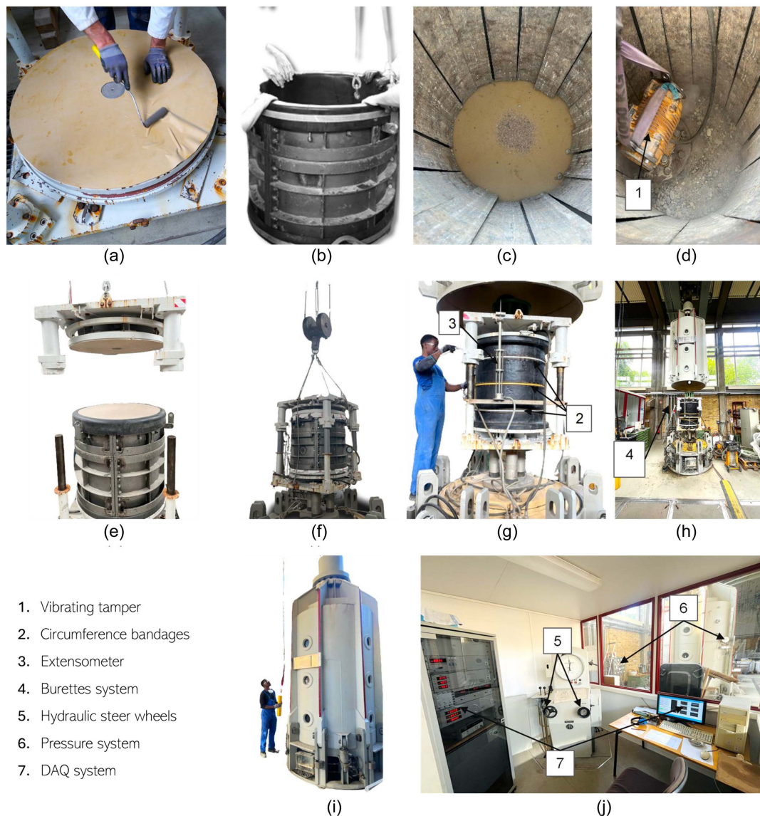
Fig. 6. Setup of L specimens: (a) adding rubber to the lubricated base platen; (b) membrane installation; (c) installing membrane protection plates and sand layer at the center to protect drainage; (d) filling the material inside and compacting; (e) adding a sand layer to level the top surface; (f) specimen transportation to the testing pedestal; (g) placing circumference bandages and vertical displacement extensometers; (h) installing the cell; (i) specimen ready for testing; and (j) data acquisition system.
