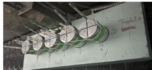
Figure 2: The setup at the γ-irradiation facility at STERIS, showing five samples, each with four alanine dosimeters to characterise the spatial distribution of dose on each side of each sample. Photo courtesy of P. Reppert.
