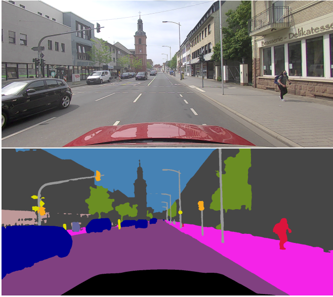
Figure 4.9: A sample image in the Opel data and its semantic segmentation mask predicted by DeepLabv3+. The hood area of the ego car is blacked out in the prediction image.
