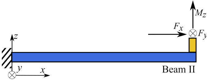
Figure 6.5: Beam II with virtual external loads at the separation point to calculate its structural stiffness.
