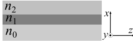
Figure 3.1: Sketch of a planar waveguide composed of three layers with different refractive indices.
