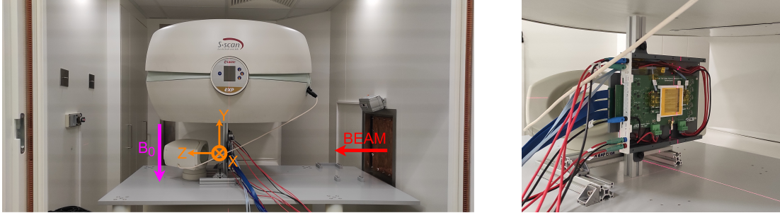
Figure 7.43.: General (left) and zoomed (right) views of the HitPix3 beam monitor demonstrator installed at the isocenter of the MRI setup at HIT. The red and magenta arrows in the general view represent the direction of the beam and static magnetic field, respectively. The orange arrows in the general view represent the axes of the demonstrator local coordinate system.
