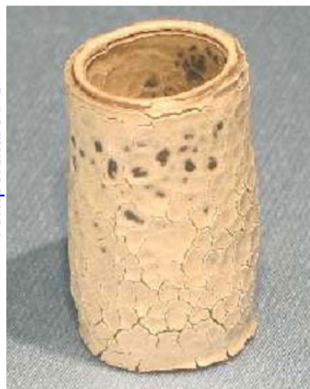
Fig. 1 Thermogravimetric curves and temperature evolution during oxidation of Zircaloy-4 and M5 cladding materials (left). Picture of fully oxidized Zircaloy-4 sample (right)
