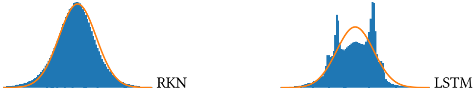
Figure 4.2.: To evaluate the quality of our uncertainty prediction we compute the normalized error \frac{x^{(j)} - \hat{x}^{(j),+}}{\sigma^{(j),+}} for each entry j of \mathbf{x} for all time steps in all test sequences. This normalized error should follow a Gaussian distribution with unit variance if the prediction is correct. We compare the resulting error histograms with a unit variance Gaussian. The left histogram shows the RKN, the right one the LSTM. The RKN perfectly fits the normal distribution while the LSTM’s normalized error distribution has several modes. Again we designed the smaller LSTM and GRU to have roughly the same amount of parameters as the RKN.
