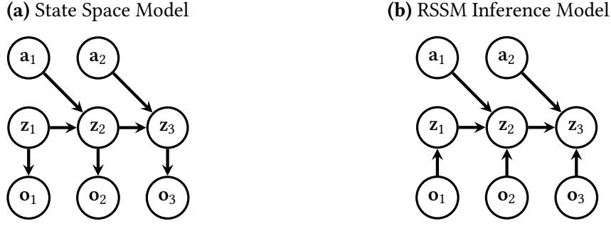
Figure 5.1.: (a) State space model, serving as the generative model throughout this work. (b) Graphical Model underlying the RSSM (Hafner et al., 2019) inference scheme. In contrast to the generative SSM, the direction between observations and latent states is inverted. These independence assumptions result in a simplified inference and subtle effects on model learning.
