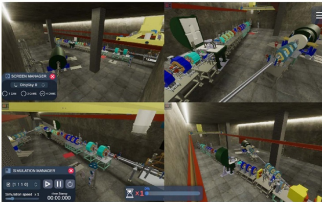
Figure 29. Operator view of the RH operation through the viewing system in VR simulations. Reproduced from [17]. CC BY 4.0.
