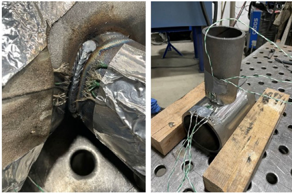
Fig. 1 Measurement of the t_{8.5} time with type K thermocouples [4]
