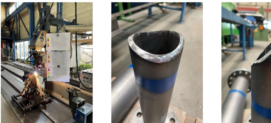
Fig. 5 Cutting (3D intersection curve + weld preparation) of the CHS with CNC-controlled plasma cutting robots [4]
