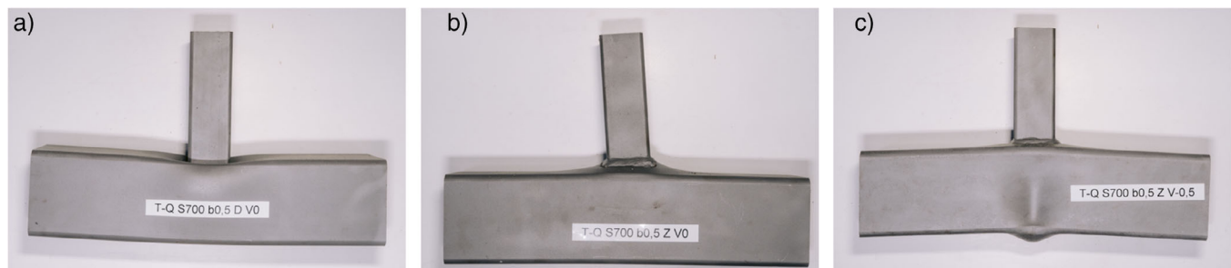
Fig. 9 Failure mechanisms depending on the type of loading [1]: a) no preload and compressive stress on the brace, b) no preload and tension stress on the brace, c) compression preload and tension stress on the brace
