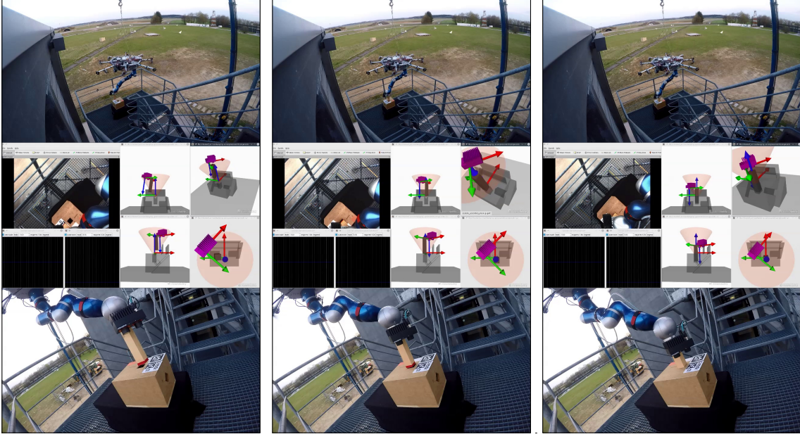
Figure 8.16.: Qualitative results for peg-in-hole tasks. Left: approach phase. Middle: precise positioning. Right: successful insertion. Top: overview of the robot's remote workspace, where SAM is suspended by a crane. Middle: the operator view with live video streams, and the created VR, which displays four different view points simultaneously, and provides haptic guidance in both position and orientation. Bottom: close view on the robot's workspace. With the proposed VR-based system, we achieve precise peg-in-hole task with the robot in outdoor environments.
