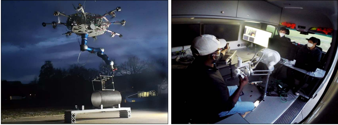
Figure 8.1.: Left: the cable-Suspended Aerial Manipulator, dubbed SAM (Sarkisov et al., 2019) during field experiment. Right: a ground station where an operator remotely controls the robotic arm through a haptic interface. In real world applications of bilateral teleoperation, the operator is often remotely located without visual contact to the robot.
