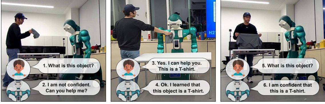
Figure 6.1.: Imagine a robot encountering an unseen object, e.g., trained for apples, but tested on a T-shirt. This problem of distributional shifts induce learning algorithms to fail. We propose an active learner with Deep Neural Networks (DNNs). With our system, the robot queries a human whenever the model is uncertain, and adapt itself to reduce that uncertainty. Such capabilities can improve the robustness of DNN-based semantic perception by coping with distribution shifts.
