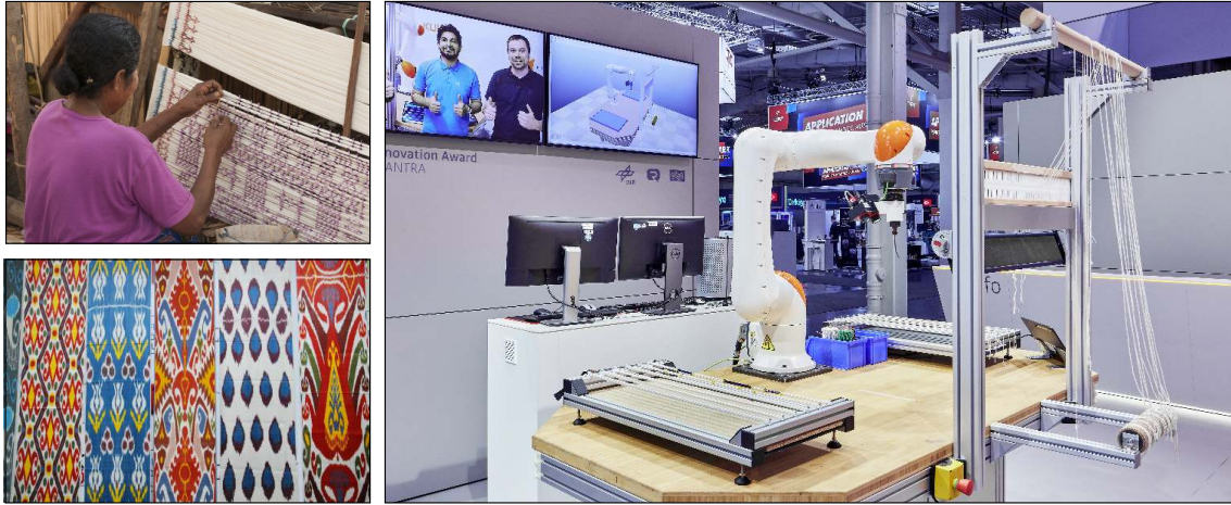
Figure 10.1.: Left: visualization of ikat, which is a preparatory phase for traditional textile manufacturing in Asia. The resulting fabric contains many patterns, which is marked and dyed by a craft person. Right: the system Yantra at Hannover Messe. Yantra supports the craftsmen by preparing the hand-loom and mark or paint the yarn threads with a collaborative robot.
