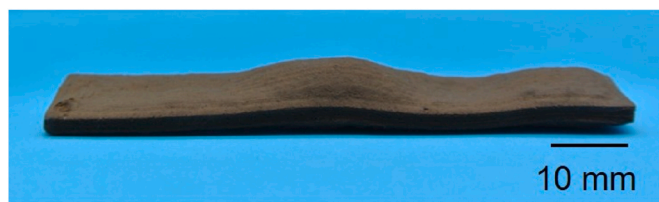
Fig. 6. 3D printed plates after debinding at temperatures of up to 220 °C with a heating rate of 5 K/min, initial printing parameter.
