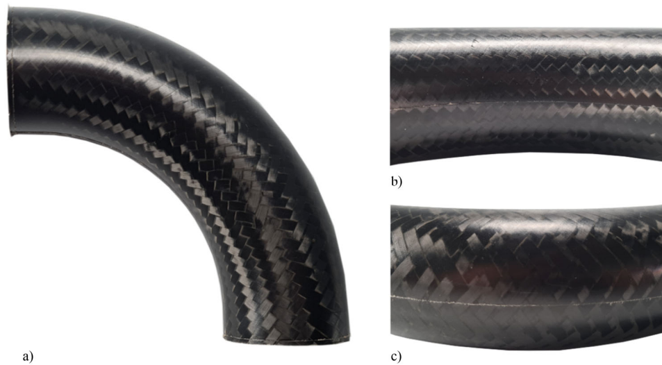
Figure 17. Curved demonstrator manufactured by BAM (a); Detailed view of the intrados (b); Detailed view of the extrados (c).
