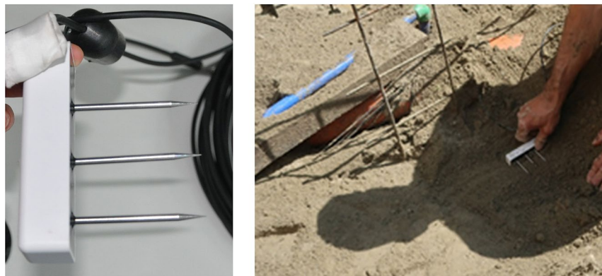
Fig. 10 Installation of the soil moisture sensors at a close distance from the planar trench collector.
