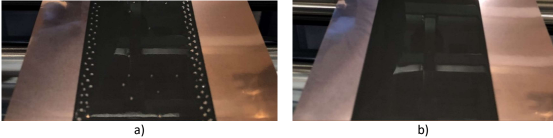
Figure 4-12: Inline photographs of the roll-to-roll coating experiments, web's direction from bottom to top; a) coating outside stable operating window with visible air entrainment; b) coating within the stable operating window.
