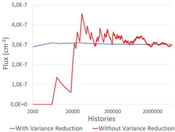
Figure 52. Evolution of the total neutron flux and relative error behind a 10 cm thick copper slab irradiated by a perpendicular 9 MeV deuteron beam, normalized by source particle.
