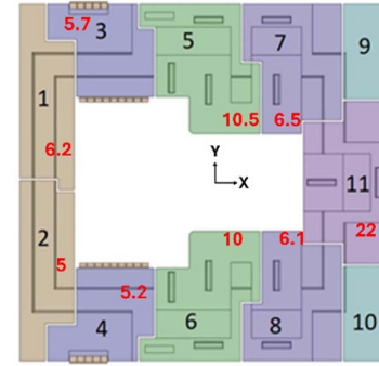
Figure 5. Layout of all the RBSBs providing the cavity for the TC liner. Red highlighted values are the integrated nuclear heats (kW) per each RBSB.
