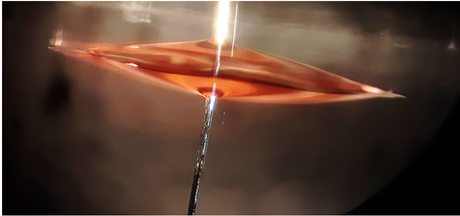
Figure C.2: Top view of a fibre tip being cleaned with a drop of First Contact cleaning polymer. The reflection of the fibre in the drop surface is used for alignment.
