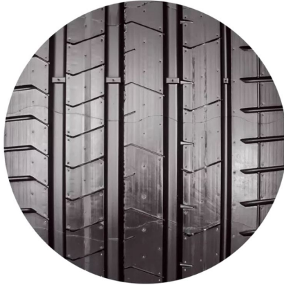
Figure A.4: Tread profile of the summer tire examined.
