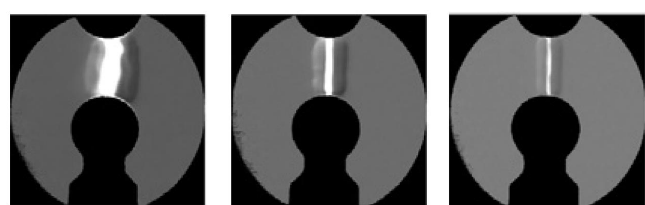
Fig. 3: Schlieren image of the spark ignition for \alpha = 0, \alpha = 0.05, \alpha = 0.1 [3]
