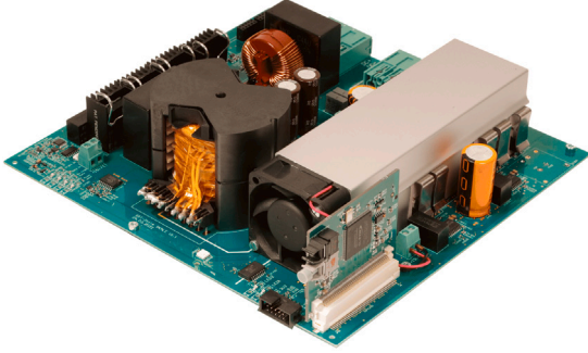
Fig. 10. Hardware of the power module with a DAB stage and the CHB cell.
