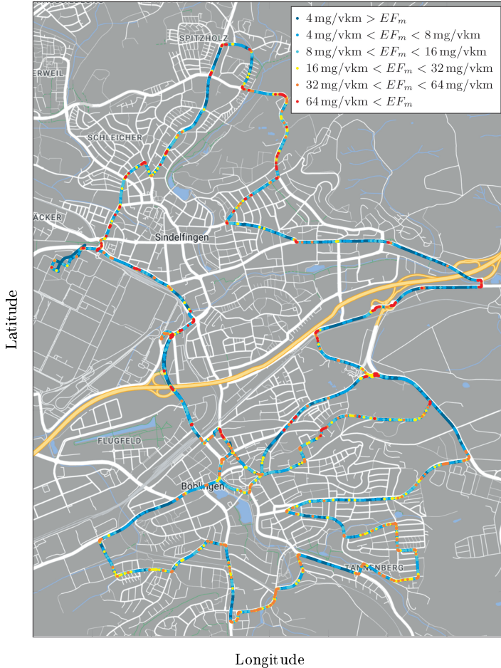
Figure 6.7: Prediction of the emission factor of tire–road PM for a luxury-class vehicle driving with summer tires depending on the location for the urban route profile assuming an SRT value of 60.
