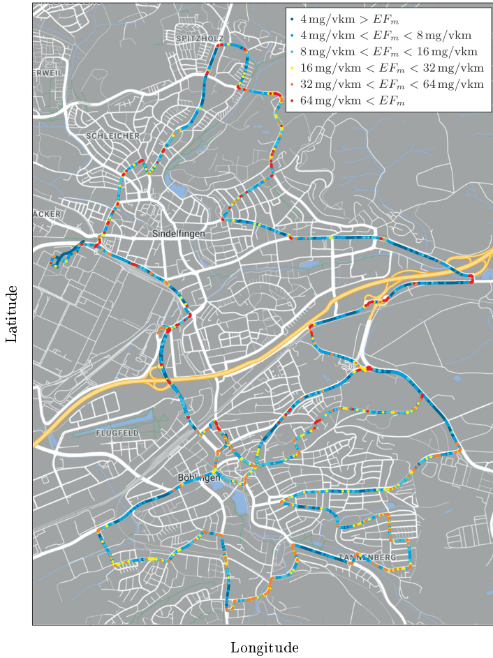
Figure A.24: Prediction of the emission factor of tire-road PM for a luxury-class vehicle driving with summer tires depending on the location for the urban route profile assuming an SRT value of 60 (identical with Figure 6.7).
