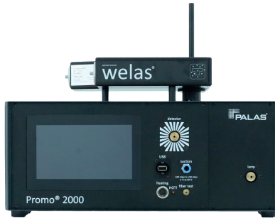
Figure 3.4: Optical aerosol spectrometer system PALAS Promo 2000 with aerosol sensor welas 2500 [94].
